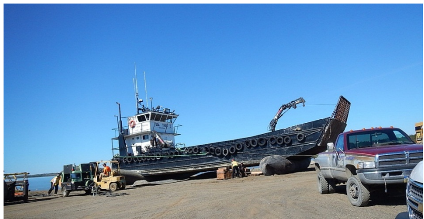
Hauling out a landing craft in Homer using airbags.
